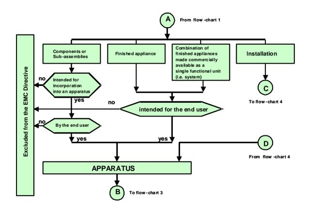
For guidance on the applicability of the EMC Directive to components, sub-assemblies, finished appliances, combinations of finished appliances and mobile installations the reader is referred to section 1.2, which defines the scope of apparatus. For fixed installations the reader should consider section 1.3.
